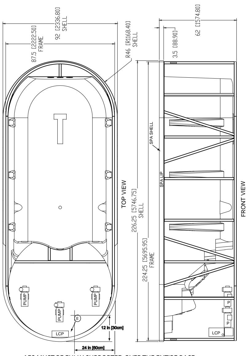
AFS MUST BE FULLY SUPPORTED OVER THE ENTIRE BASE. REFER TO D1 DOC-138 FOR INSTALLATION DETAILS.
