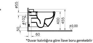
\*Additional pipe may be required as to wall thickness
